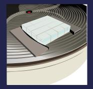
ELECTROMAGNETIC CHUCK Magnetic blocking is often used to hold non-magnetic parts in place.
