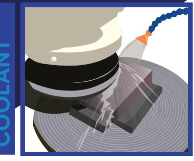
Although abrasives tend to take center stage when it comes to grinding process optimization, coolant is another extremely important factor in obtaining consistent results. When it comes to your specific process, remember:
