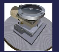
CUSTOM FIXTURES Fixtures built for a specific part or purpose such as tilting the part on the table.
